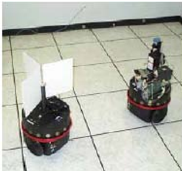
Figure 5.6: Robot tracker: The observed robot with white target on the left and the observing robot with the laser range finder on the right. Presented in [Sim 01].
