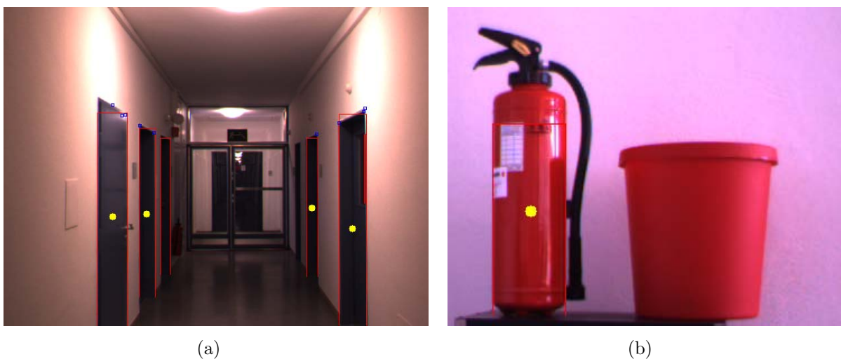
Figure 6.20: Interesting classification cases in the result of feature extractor algorithm: (a) a mismatch of the feature correspondence of the third door left in both cameras and (b) the same color as a valid feature, but different geometry and dimension
