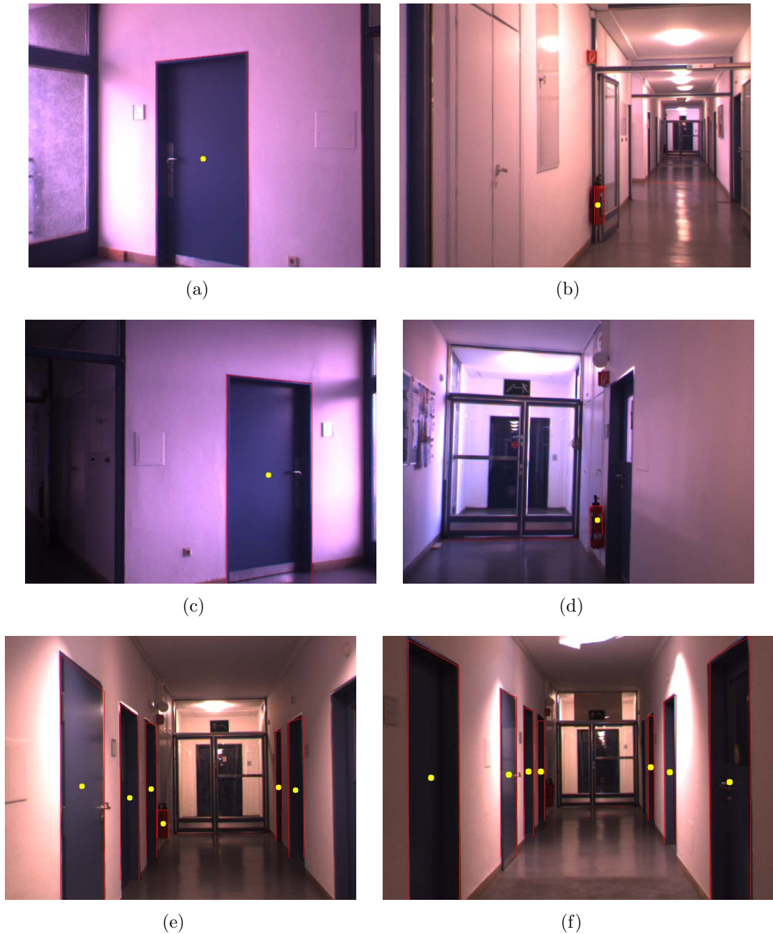
Figure 6.21: Results of feature extractor algorithm with different conditions: (a), (b), (c) and (d) The extraction process during the day at different positions, (e) and (f) the extraction process during the night with different types of features in one picture.
