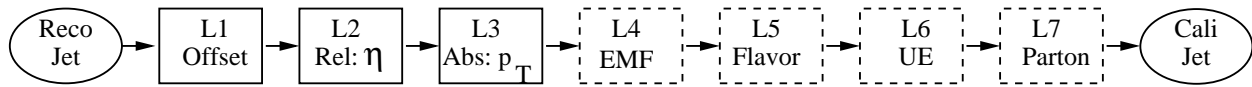
Figure 6.2: Schematic overview of the factorised multi-level jet correction in CMS. Starting with an uncalibrated calorimeter jet, several subsequent corrections can be applied. In this scheme, required correction levels are indicated with solid boxes [120].
