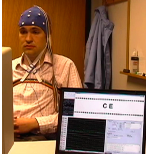
Figure 7.1: The demo setting. The laptop screen shows the hypothesis of the last 2 recognized words, which are "C" and "E"
