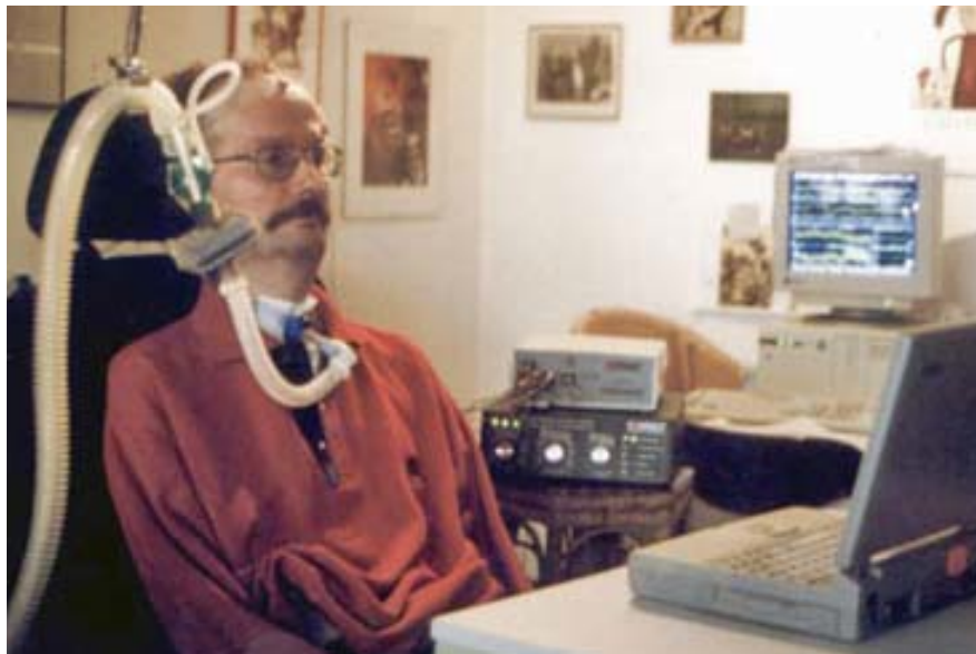
Figure 1.1: Locked-In patient using the Thought Translation Device[1] to control a computer
