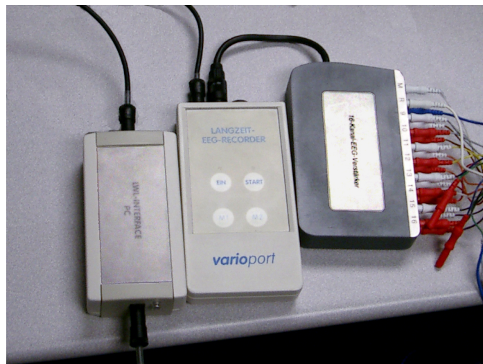
Figure 4.5: From left to right: optical waveguide, computer interface, amplifier
