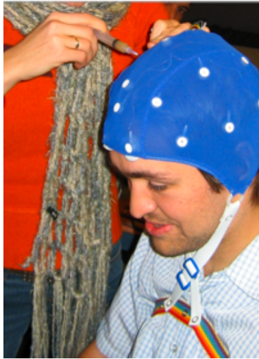
Figure 2.7: Electro-Cap being filled with a conductive gel
