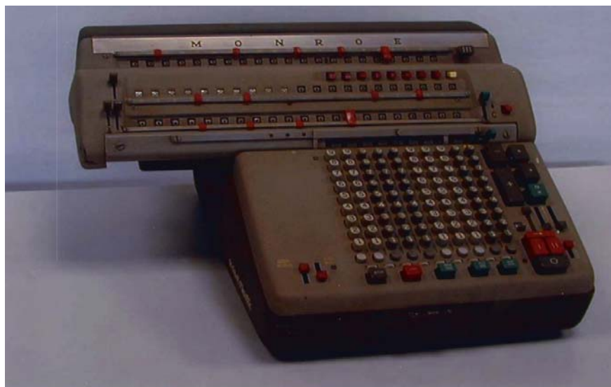
MONROE, Modell MONROMATIC ASMD (1956), von Monroe Calculating Machine Company, Inc., Orange, New Jersey, USA. Addition, Subtraktion, Multiplikation, Division, Multipliziere und Akkumuliere
