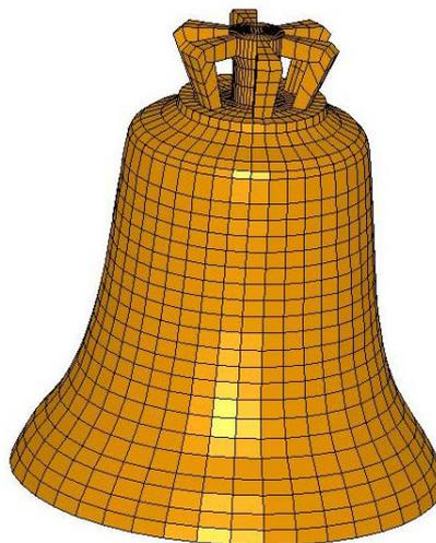
**Figure 2.** Discretized model of the carillon bell
