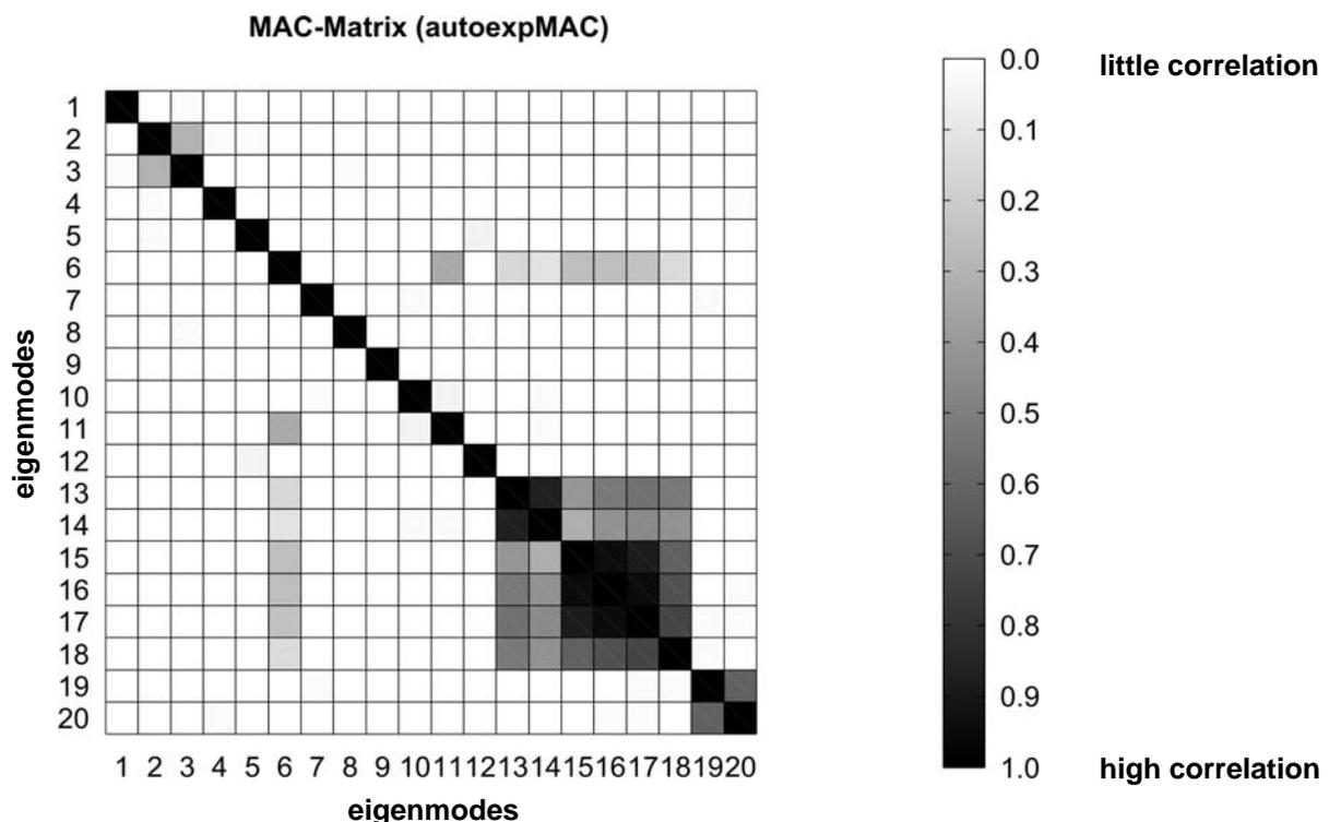
**Figure 4.** Auto MAC matrix of experimental eigenmodes
