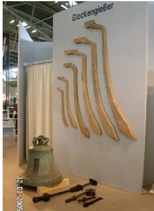
Figure 2 Different clappers, bell with crown and different cross sections of bells (bell ribs); from bell founder Perner, Passau, Germany
