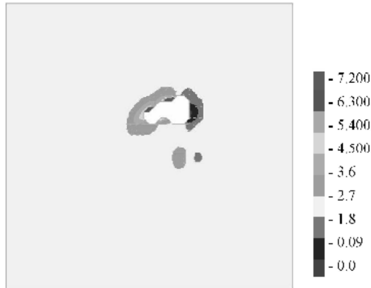
Fig.12. Pressure distribution in the fluid.
