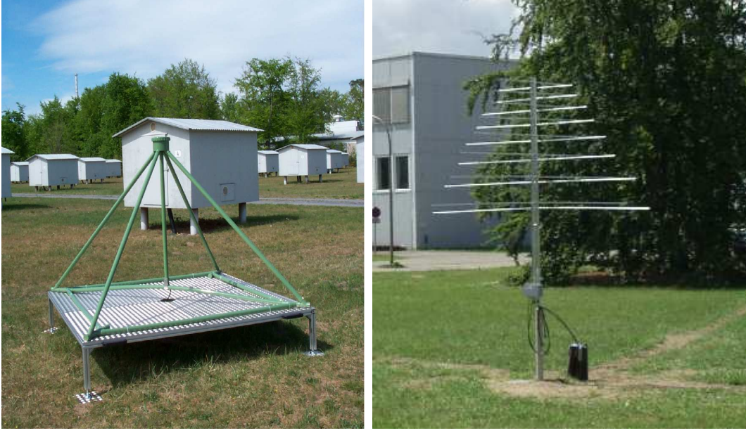
Figure 3.1: Left: LOFAR prototype antenna. Right: LOPES STAR type, LPDA. Inside the KASCADE-array the LOPES antennas are installed between the detector station. The pyramid geometry determines the receiving characteristics of the antenna. At two opposite sides of the pyramid the dipole antenna is placed, causing the inverted-V shape.
