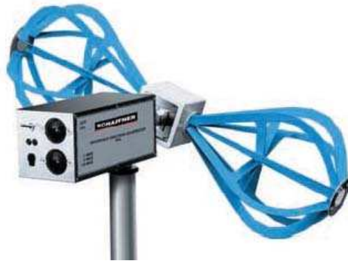
Figure 4.3: The VSQ 1000 from Schaffner consists of the signal generator RSG 1000 and the biconical antenna DPA 4000. The total length of the biconical antenna is 40.5 cm (image courtesy of Schaffner).
