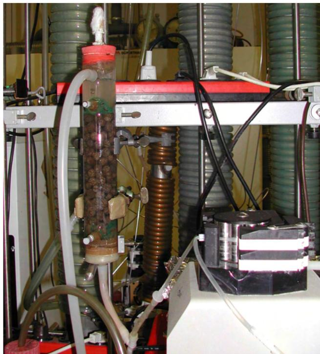
**Picture 1: Aerobic fixed bed reactor for phenolic wastewater**
