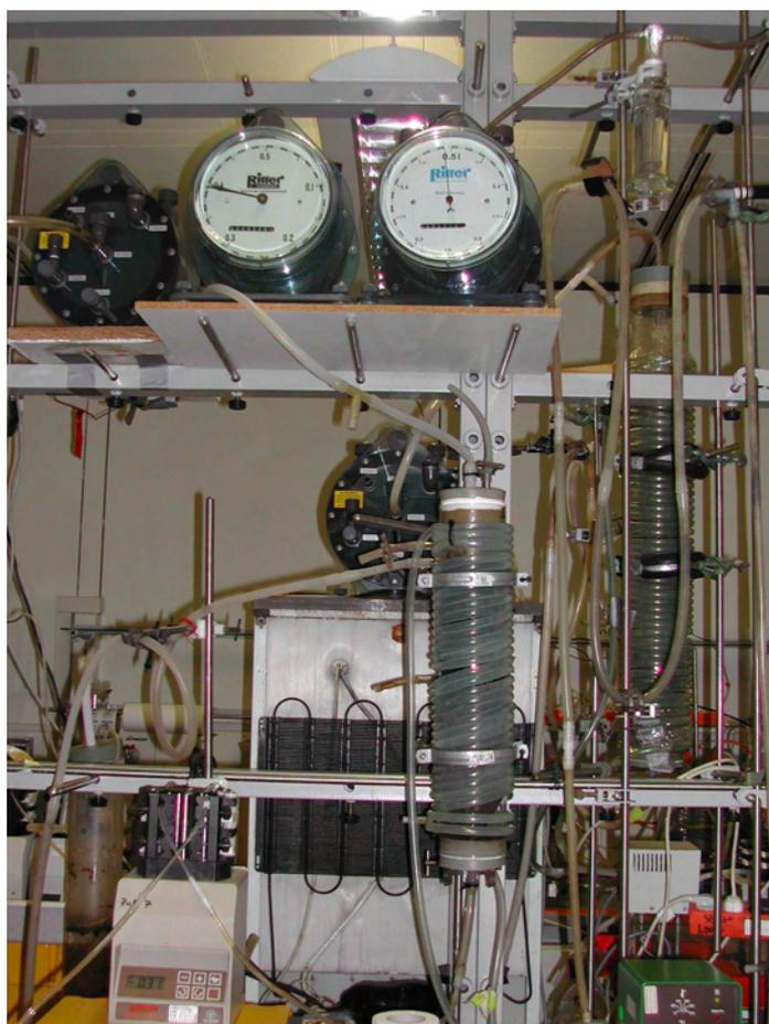
**Picture 9: Anaerobic suspended bed reactor for 2-CP degradation**
