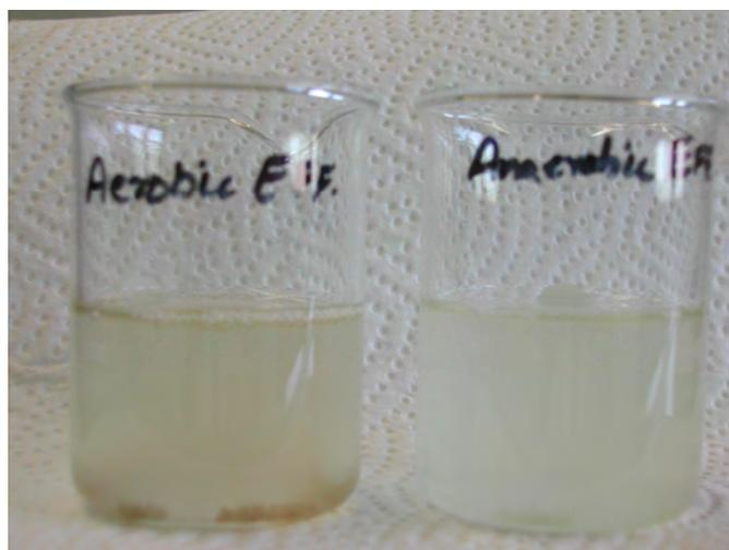
**Picture 5: A comparison between aerobic and anaerobic fixed bed effluents**
