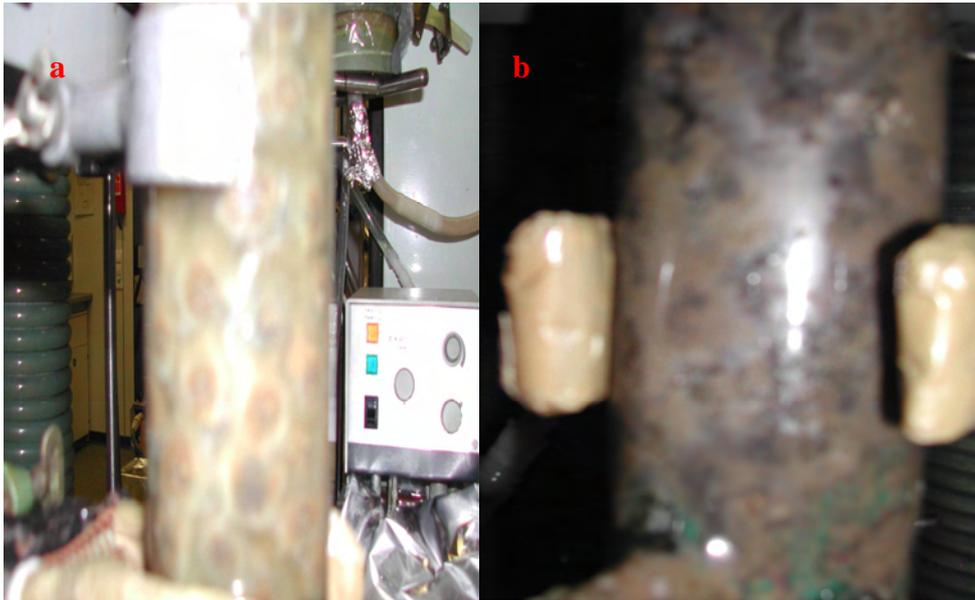
**Picture 3: Sludge growth on aerobic fixed bed 3 weeks (a) and 6 weeks after reactor start-up (b)**
