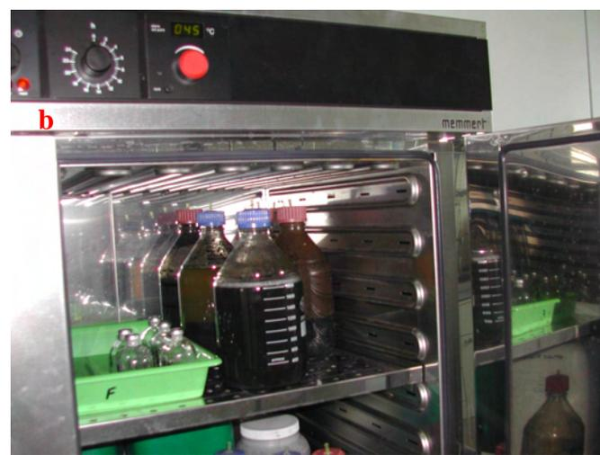
**Picture 11: Anoxic batch (a) and acclimatisation of anaerobic sludge to 2-CP under batch conditions (b)**
