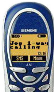
Figure 10.1: An incoming one-way phone call can be recognized from the caller ID, on any mobile phone.
