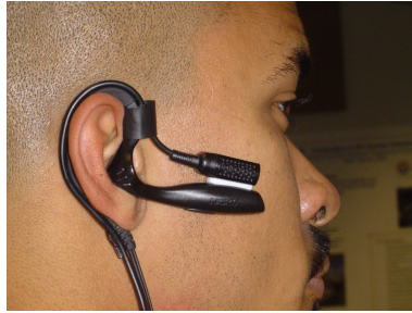
Figure 8.2: Initially, acoustic signals were captured by a wearable microphone.
