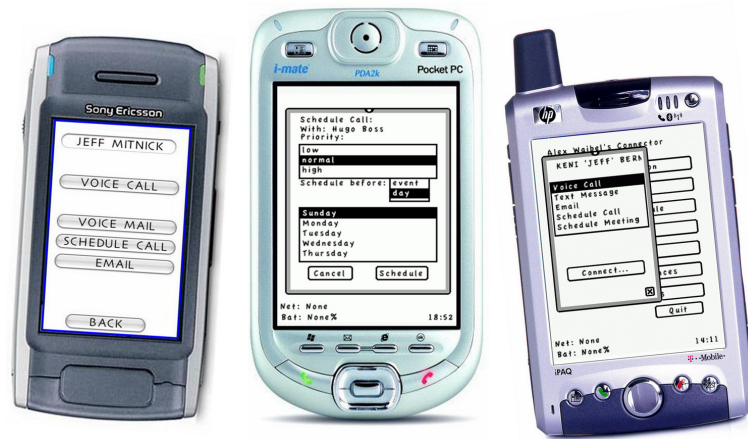
Figure 8.4: Three generations of smart Connector Phones: Sony Ericsson P900, i-mate PDA2K GSM/GPRS Pocket PC, and HP iPAQ h6315 .
