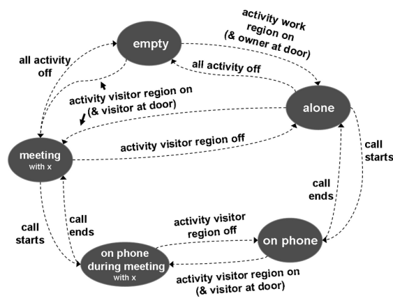
Figure 7.5: This finite state machine illustrates office activities and possible transitions between them.
