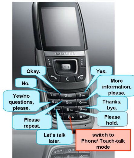
Figure 11.1: With Touch-Talk, receivers could answer incoming calls without speaking aloud by pressing keypad buttons, which would literally make the phone speak for them.
