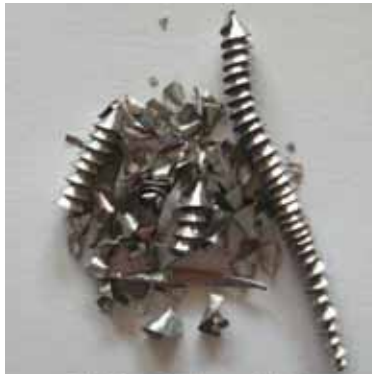
f_z = 0,025 \text{ mm/Schneide}; v_c = 100 \text{ m/min}
