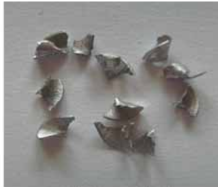
f_z = 0,150 \text{ mm/Schneide}; v_c = 350 \text{ m/min}
