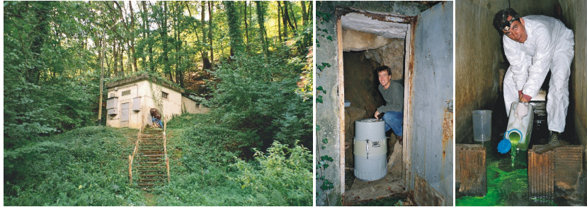
Fig. 4.83: Moulinet Spring (left), sampler at Moulinet Spring (middle; photograph: N. Goldscheider) and injection of the fluorescent tracer into the concrete-encased swallow hole (right; photograph: M. Pronk).
