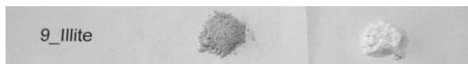
Figure 6.21 Colour of the material before and after acid treatment (5 M H 2 SO 4 at 80 °C).
