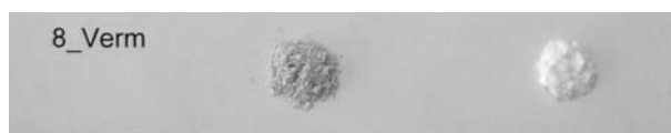
Figure 6.15 Colour of the material before (left) and after (right) acid treatment (5 M H 2 SO 4 , 80 °C).
