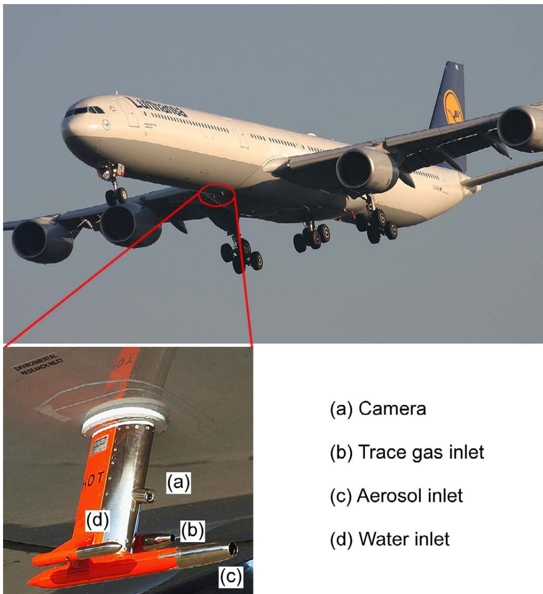
Figure 1.8: Lufthansa Airbus A340-600 “Leverkusen” (Photograph © Florian Kondziela, www.airliners.net ). The aircraft is equipped with an inlet system located at the lower side of the fuselage in front of the wing section. The inlet system provides ports to sample trace gases (b), aerosols (c), as well as both total and gas-phase water (d). A forward facing camera system (a) is used to record videos of the flights for better linkage of weather conditions and measurement data. The inlet system is heated to maximize time response and to evaporate cloud droplets or ice particles. The CARIBIC container with the various instruments is located in the cargo bay of the aircraft above the inlet system.
