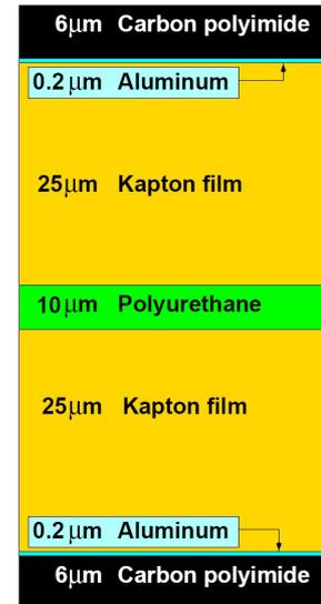
**Figure 3.20:** Cross section of the straw tube walls.
