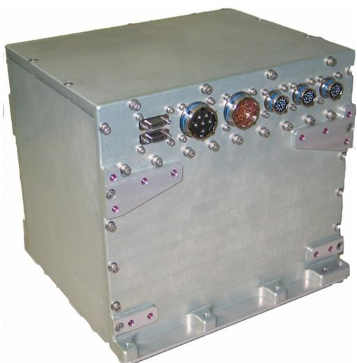
**Figure 4.19:** Photo of the UPD box. Visible is the right main wall with the 28 V supply and the HV as well as digital 3.3 V output connectors.
