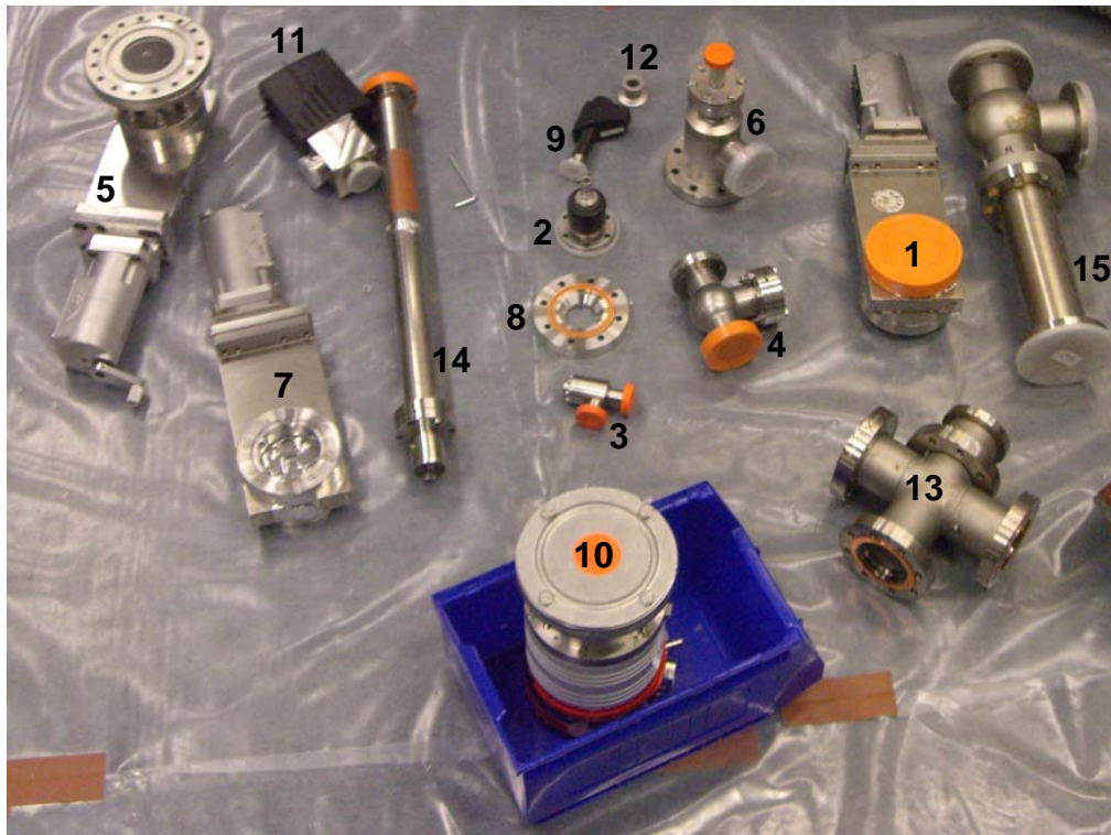
Figure 6.6: Disassembled components. Items: (1) VAT CF63 gate valve (HV006); (2) cold cathode pressure gauge (RP002); (3) VAT CF16 angle valve (HV022); (4) CF40 T-piece (connection to item no. 2); (5) VAT CF63 gate valve (HV061); (6) CF63-CF40 T-piece; (7) VAT CF63 gate valve (HV005); (8) CF60-40 transition flange; (9) Pirani pressure gauge (RP003); (10) turbomolecular pump (VP061); (11) KF25 automatic valve (AV061); (12) KF16-KF25 transition flange; (13) CF63 cross piece; (14) gold plated detector chamber; (15) gold plated RGA chamber and T-piece of the Detection System. A PID is available in appendix D.
