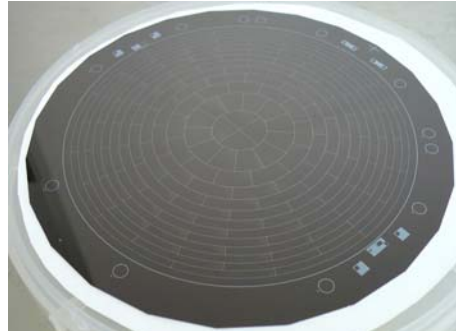
Figure 2.8: Prototype of the Focal Plane Detector. [Doe08]
