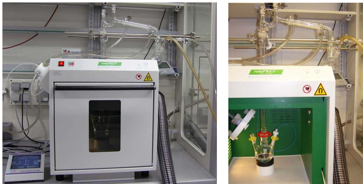
Figure 1. Experimental set-up of microwave-assisted polyol synthesis.
