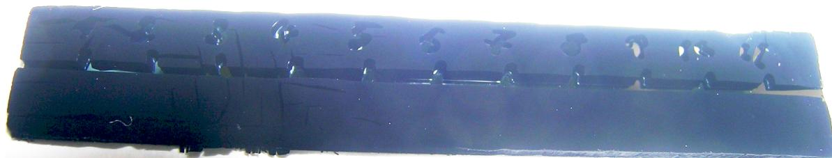
**Figure 4.5:** 6 x 1 cm chip covered with vertically aligned nanotubes. The chip was prepared with 10 nm of  $\text{Al}_2\text{O}_3$  and an iron gradient from 1 to 0.2 nm. Numbers were written with a pen on the chip before sputtering and removed with acetone before CVD growth. The iron catalyst layer is thickest around 1 and decreases in height towards 11.
