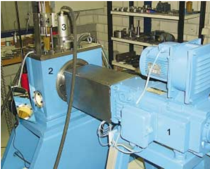
Bild 8: Kleiner Lagerprüfstand 1: Elektromotor; 2: Prüfstandsgehäuse; 3: Hydraulikzylinder; 4: Endoskopkamera Figure 8: Small bearing test bench 1: Motor; 2: Test bench housing; 3: Hydraulic cylinder; 4: Endoscope-camera
