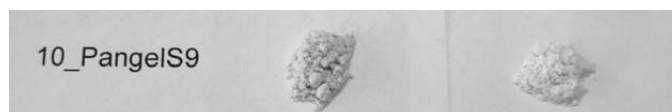
Figure 6.25 Colour of the material before (left) and after (right) acid treatment (5 M H 2 SO 4 , 80 °C).
