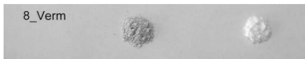
Figure 6.15 Colour of the material before (left) and after (right) acid treatment (5 M H 2 SO 4 , 80 °C).
