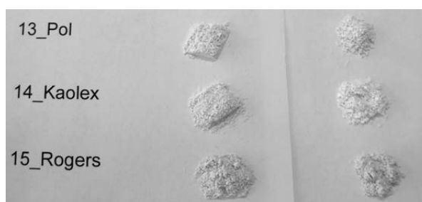
Figure 6.30 Colour of the material before (left) and after (right) acid treatment (5 M \text{H}_2\text{SO}_4 , 80 °C).
