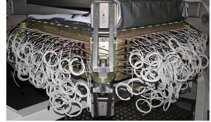
Figure 3.18: The ECAL before the integration into AMS-02.
