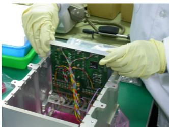
The S9011AU board during the insertion into the UPD box.
