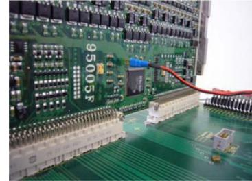
Figure 5.2: *UDR2 test backplane solid state fuse test. Test points on the UDR2 and UPSFE boards allow to insert a load into the digital circuit in order to test the correct switching of the solid state fuses on the boards.*
