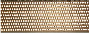
Figure 3.15: *ECAL fibers embedded in 640 kg of lead arranged in 18 layers.*
