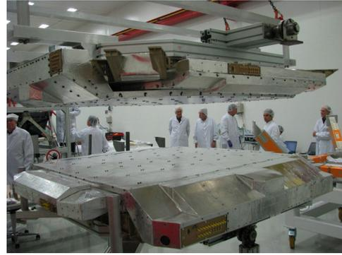
Figure 3.13: *Picture of the assembled upper and lower ToF.*
