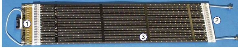
Figure 3.20: A TRD straw tube module. The 16 tubes are connected to the  $Xe/CO_2$  gas circuit by a manifold (2). On the opposite side the tube end board (1) is attached, which connects the high voltage and decouples the signal by 16 capacitors from each straw tube. Additional carbon fiber stiffeners (3) are glued between the tubes.
