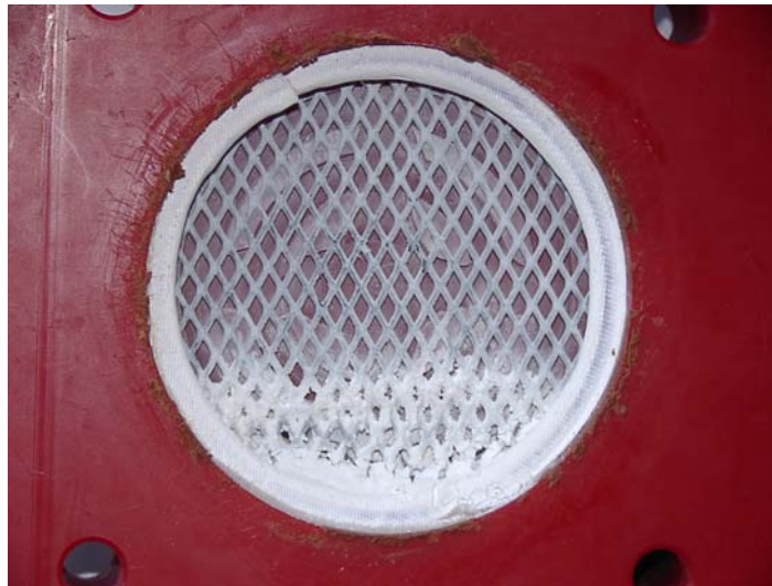
Fig. 5.40: Cathode after the electrokinetic experiment coupled with hydraulic gradient from anode to cathode and simulating constant ion supply (Ca/MgCl 2 _Z2).
