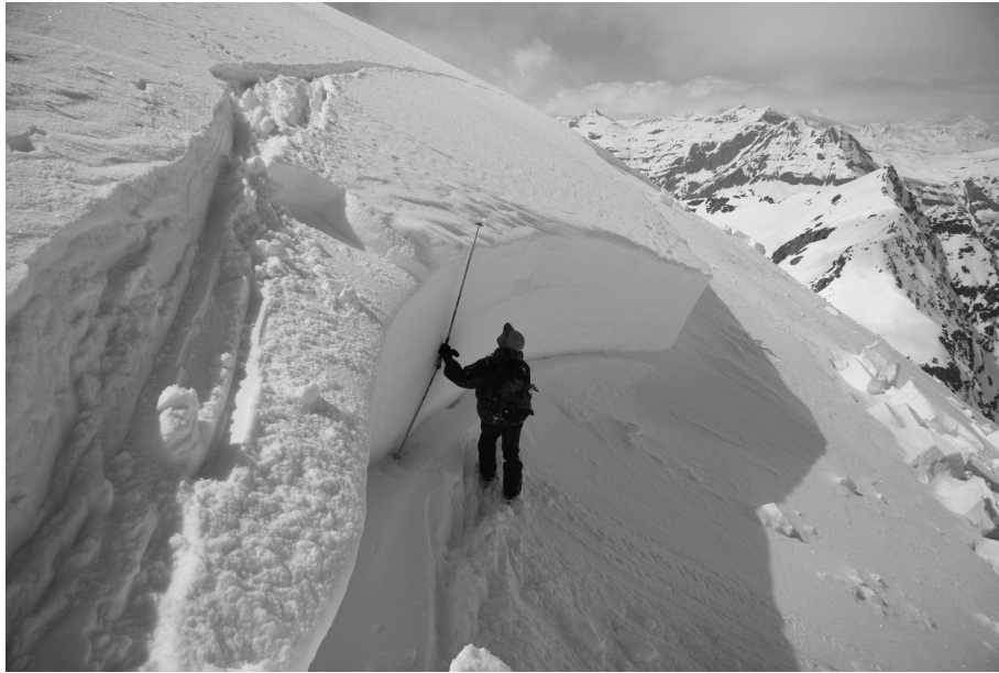
Figure 1.1: Fracture pattern showing the basal fracture plane (eroded) and the peripheral wall. This slab avalanche of exceptional size released spontaneously at Glacier du Vallonnet, France, on April 4 2007. The slab was over 2 m thick. Photo: A. Duclos, www.data-avalanche.org .
