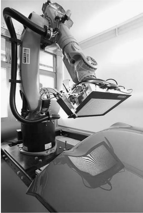
**Fig. 1** Compact, robot-based sensor head for recording of light map and optical flow data
