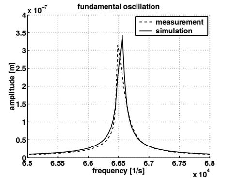
Figure 2: Comparison of the fundamental amplitudes (simulation / measurement)
