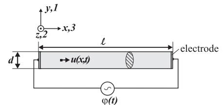
Figure 1: Model of the piezoceramic rod
