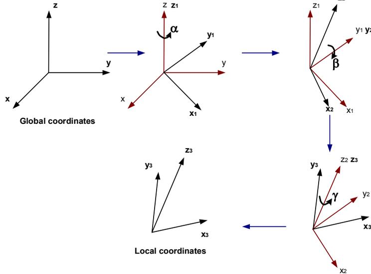
Figure 5: Coordinate transformation by using Euler angles ZYZ convention
