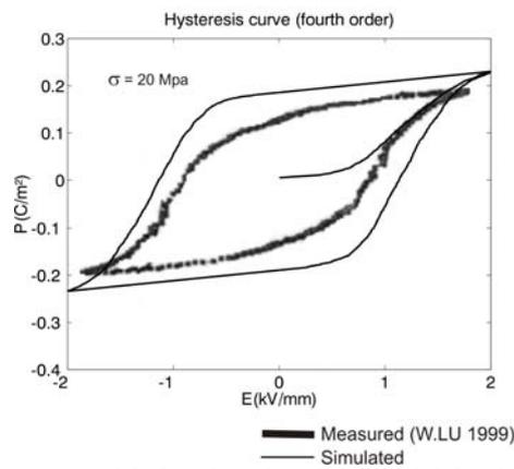
Figure 13: Hysteresis curve with fourth order polynomial for the probability function.
