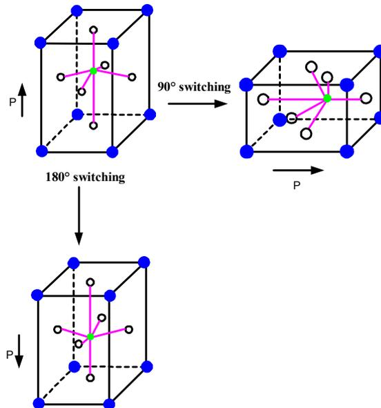
Figure 3:  $90^\circ$  and the  $180^\circ$  switching in the lattice structure of perovskite type tetragonal element
