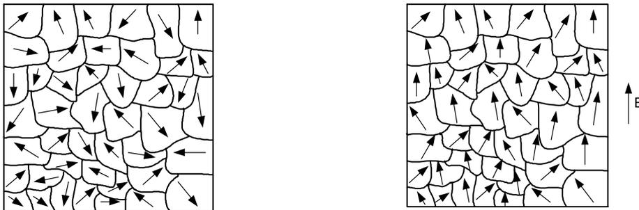
Figure 2a : Randomly oriented grains (unpoled case) Figure 2b : Fully poled grains in electric field direction
