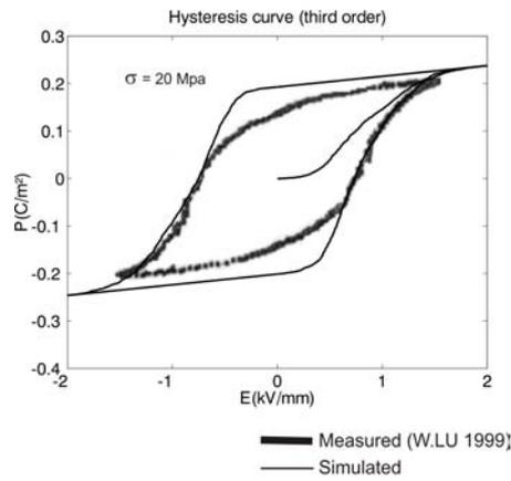
Figure 12: Hysteresis curve with third order polynomial for the probability function.
