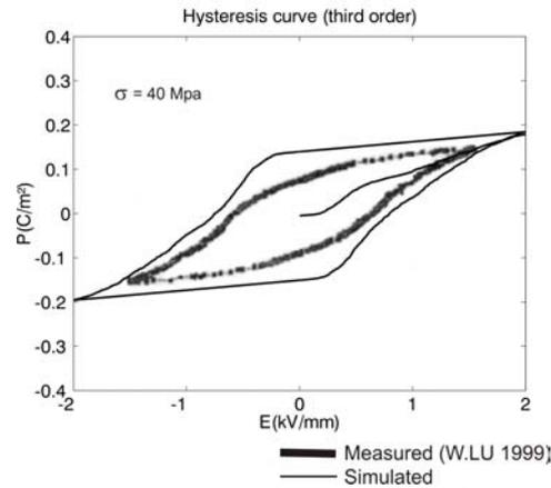
Figure 14: Hysteresis curve with third order polynomial for the probability function.
