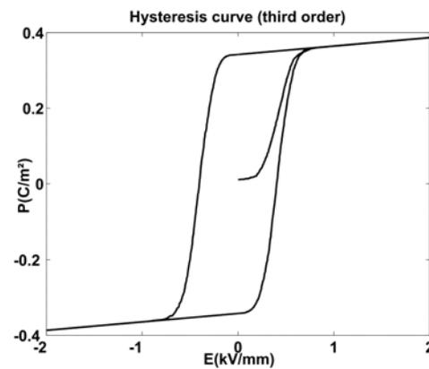
Figure 7: Hysteresis curve with third order polynomial for the probability function.
