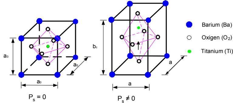
Figure 1: Lattice structure of cubic and tetragonal elements ( $\text{BaTiO}_3$ )
