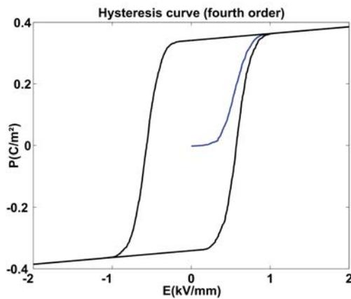
Figure 8: Hysteresis curve with fourth order polynomial for the probability function.
