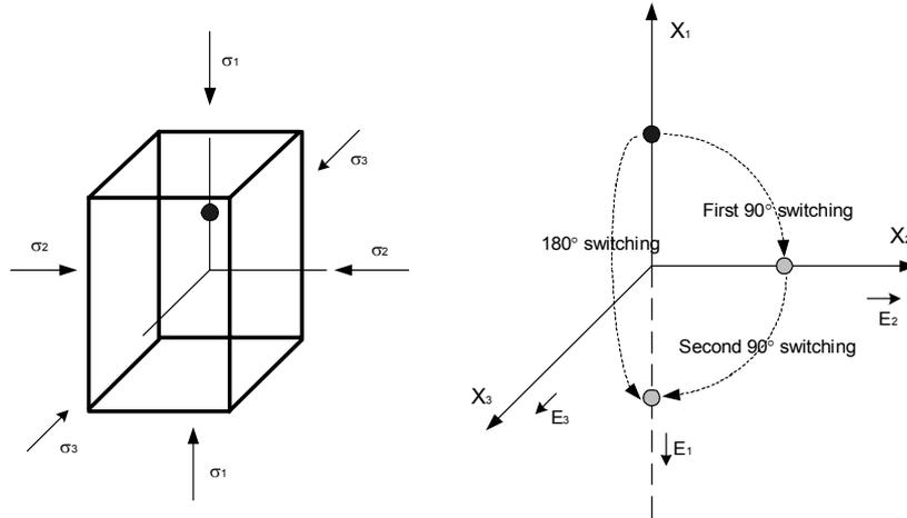
Figure 10: Lattice structure under constant compressive stress with electric field and switching possibilities
