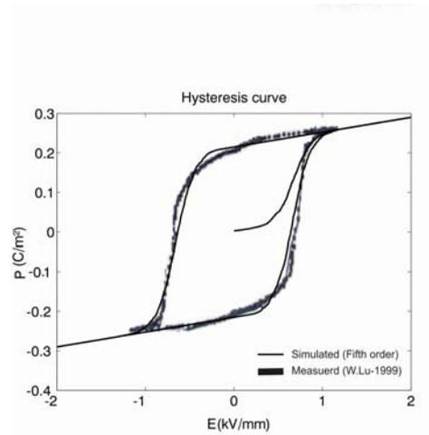
Figure 9: Comparison between simulation (fifth order polynomial for the probability function) and measured data.
