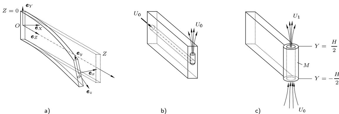
Figure 1. Bar Model, Coordinate Systems and Layouts of Fluid Jet Load.
