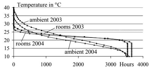
Figure 3: Cumulative frequency distributions for hourly averaged room (air) and ambient temperatures from May 1<sup>st</sup> to September 30<sup>th</sup> in 2003 and 2004. Due to the type and position of the temperature sensors, indoor air temperatures approximately represent an operative temperature. The room temperature is an average out of 4 office rooms which are exclusively cooled by passive means.
