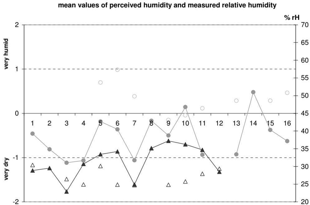
**Figure 5: Perceived humidity together with measured relative humidity (mean values of six rooms measured between 10 am and 3 pm on the day of the survey).**
