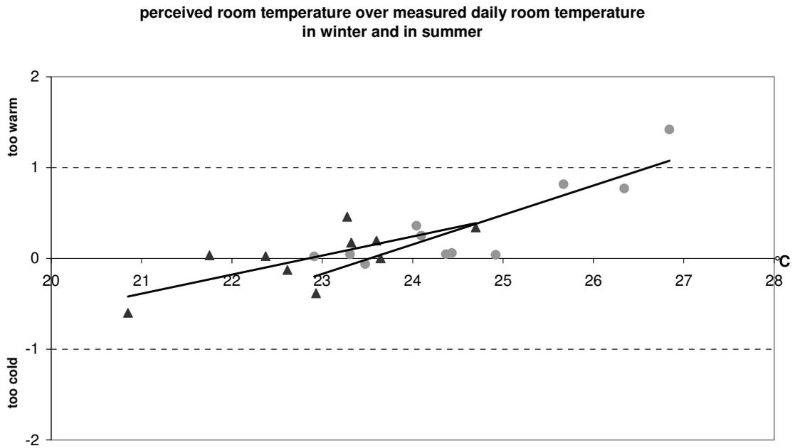
**Figure 2: Temperature rating over measured room temperature (mean values of six rooms between 10 am and 3 pm on the day of the survey) in winter (black triangles) and summer (grey spots).**
