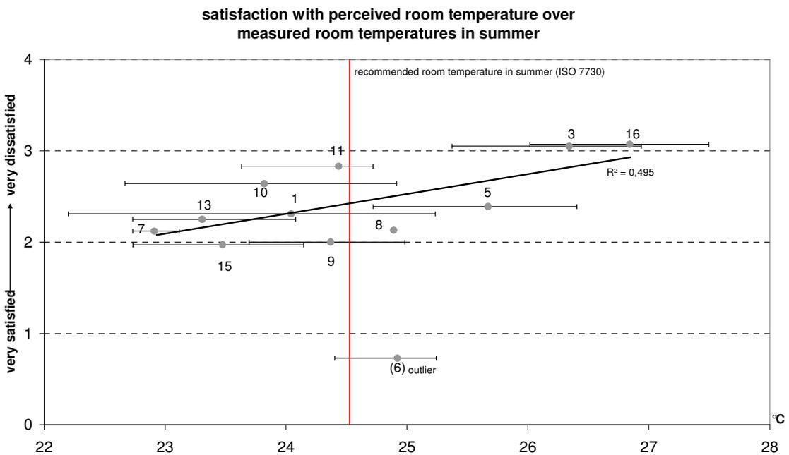
**Figure 3: Mean satisfaction vote with respect to room temperature in summer versus the measured room temperature (mean value of six rooms measured between 10 am and 3 pm on the day of the survey).**
