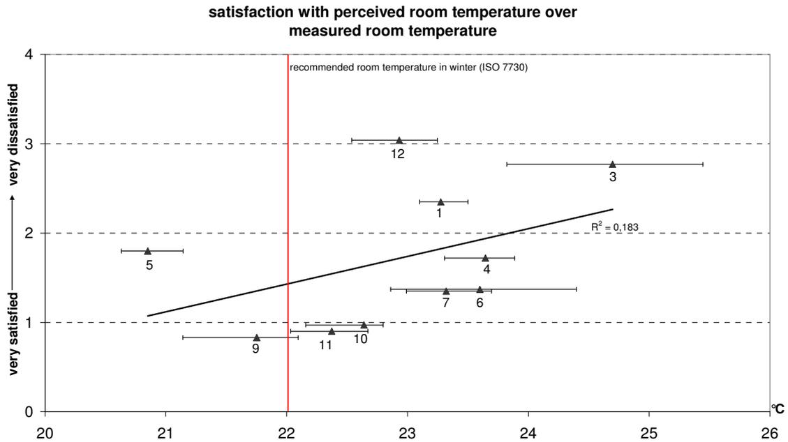
**Figure 4: Satisfaction Vote with respect to room temperature in winter over the measured room temperature (mean value of six rooms measured between 10 am and 3 pm on the day of the survey).**
