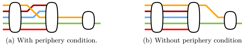
Figure 4.3: Layout of a terminus (middle vertex) with and without periphery condition. The layout without periphery condition introduces a gap between the ongoing lines (b).
