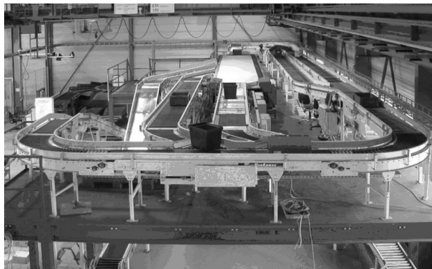
Figure 3.4: Continuous conveyors with decentralized control at the IML for researching the "Internet of Things", source: ten Hompel, Libert, and Sondhof 2006
