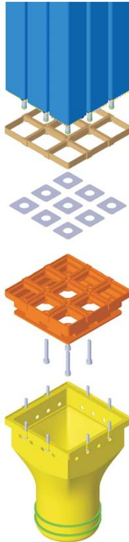
Figure 10.2: Footpiece of FA cluster with inlet orifices.
