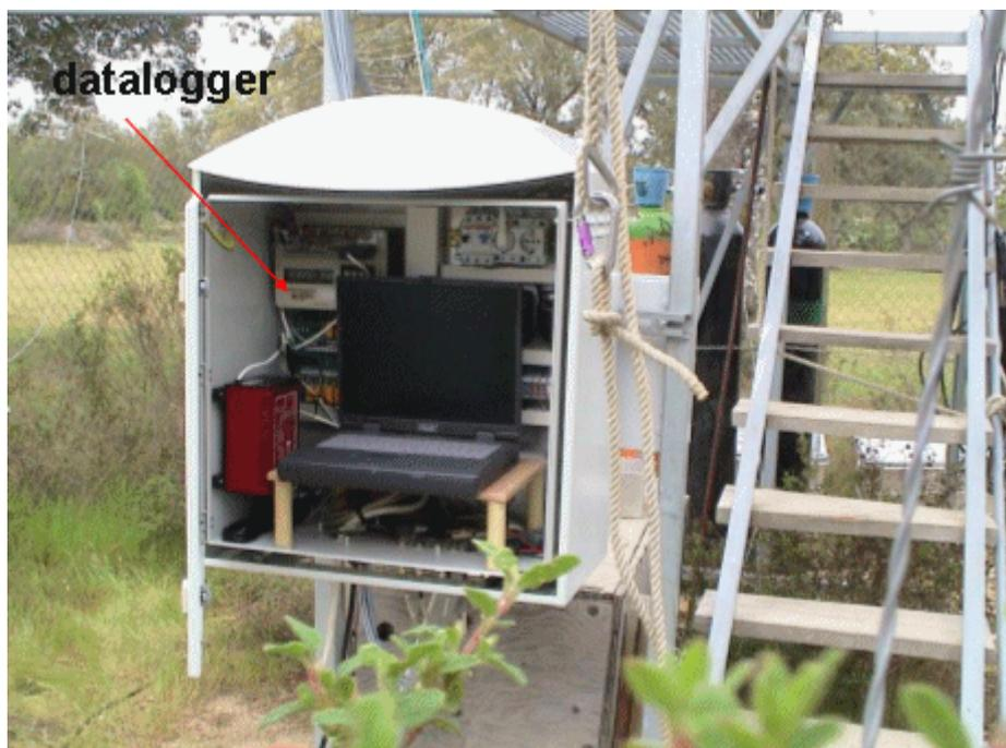
*Figure 4.17: Control unit of the station. A white painted protecting case contains the datalogger, laptop and outlets of the power supply to all instruments.*
