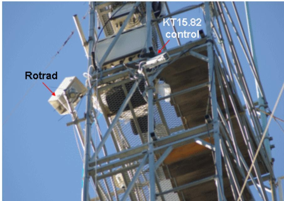
Figure 4.20: The main instruments of the station: Rotrad and KT15.82 mounted 23 m above the ground that enables measurements over the tree canopy. Both instruments are tilted, so that the construction of the tower is not in the field of view of the radiometers.
