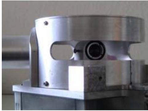
*Figure 4.12: Radiometer sensor on the rotating platform.*
