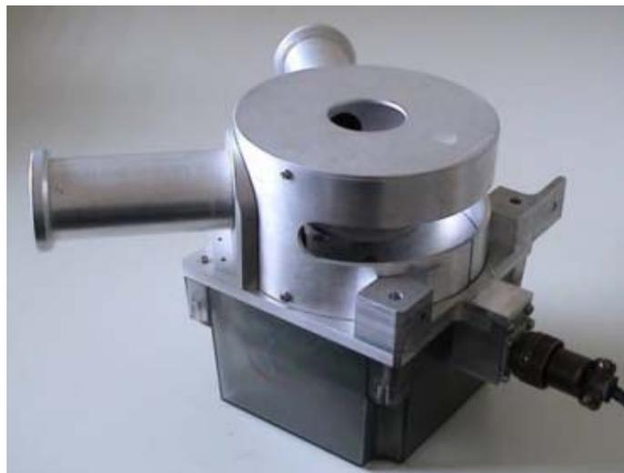
*Figure 4.11: Rotating radiometer with two black bodies for self calibration (designed by John Bennett, CSIRO).*
