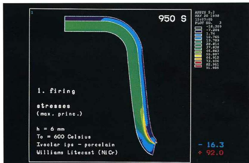
Fig 16 Distribution of residual stresses in the complete crown.
