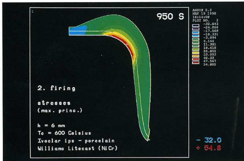
Fig 18 Distribution of residual stresses in the veneer after the second firing.
