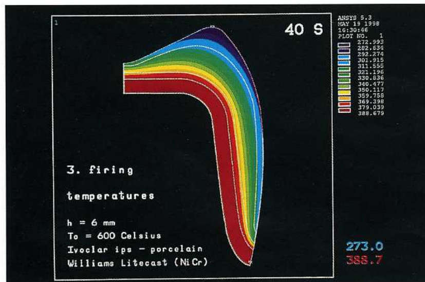
Fig 19a Temperature distribution in the complete crown for the third (dentin correction) firing 40 seconds after opening the furnace.
