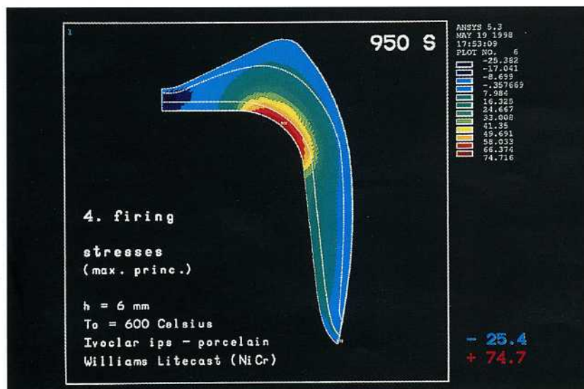
Fig 22 Distribution of residual stresses in the veneer after the fourth firing (glazing).
