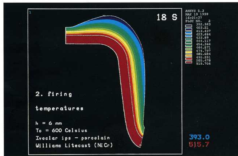
Fig 17a Temperature distribution in the complete crown for the second (first dentin) firing 18 seconds after opening the furnace.
