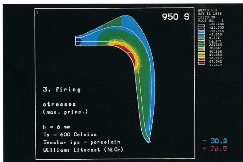
Fig 20 Distribution of residual stresses in the veneer after the third firing.
