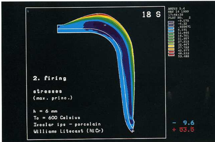
Fig 17b Accompanying distribution of transient stresses in the ceramic veneer.
