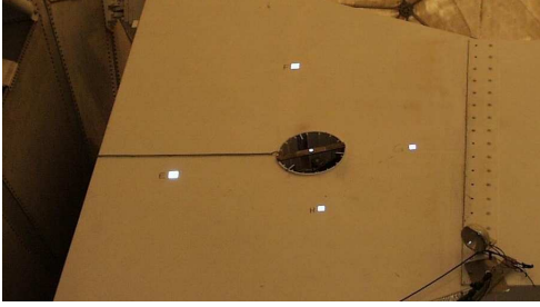
Figure 2. Target markers (2002) at the telescope cabin and at the endpoint of the elevation axis.
