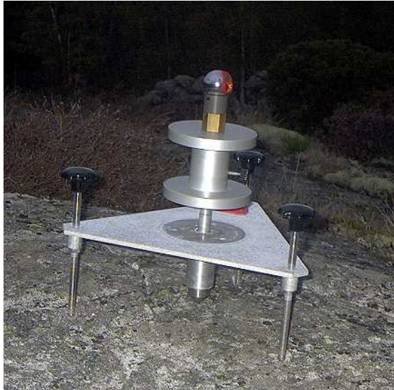
Figure 5. A small tripod equipped with a 1.5" CCR, placed on the bedrock for the traverse measurements.
