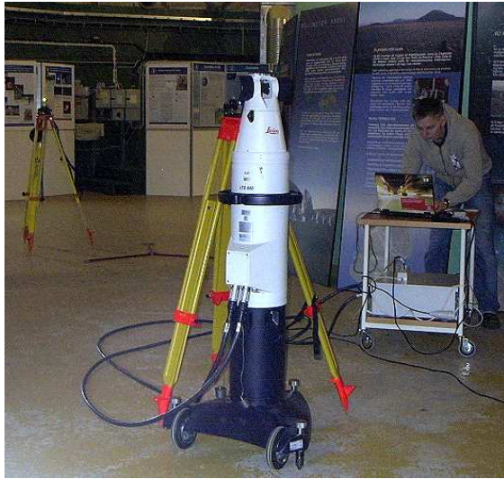
Figure 1. The laser tracker in its standard operation mode where the tracker head can move \pm 235^\circ in azimuth and \pm 45^\circ in elevation.
