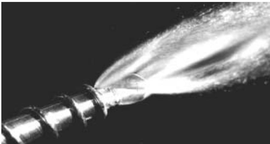
**Fig. 6:** Twist drill tip for the damageless drilling up of plugged flow paths
