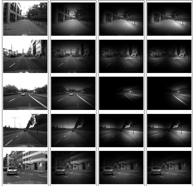
Fig. 7. In this example, the occurrence probability for a certain object category is simply a measure of local intensity contrast, i.e. regions with a low probability are black, regions with a high probability keep their original intensity value. Above, the 1 st column shows the original image, the 2 nd column shows the occurrence map of object category car , the 3 rd column shows the occurrence map of object category bicycle and the 4 th column shows the occurrence map of object category pedestrian .
