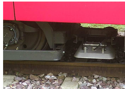
Fig. 1: Eddy current sensor system mounted on a railcar bogie.
