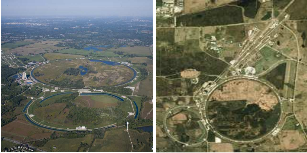
Figure 2.1: Aerial shot of the Fermilab site. Two rings of the accelerator system, the Tevatron and the Main Injector, can be seen.
