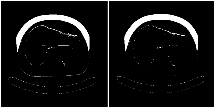
Figure 4.17: Differential images of pre-segmented CT-scans. The left image shows the result after subtracting the original segment. The right side show the same, but the segment with the overlay was moved up by one voxel. The contours of the air gaps inside the phantom are reduced clearly, which confirms the assumption of the subsided phantom. The same technique was checked for overlay 3, but the result did not improve like in the case for overlay 4, so finally the technique was only applied for overlay 4.
