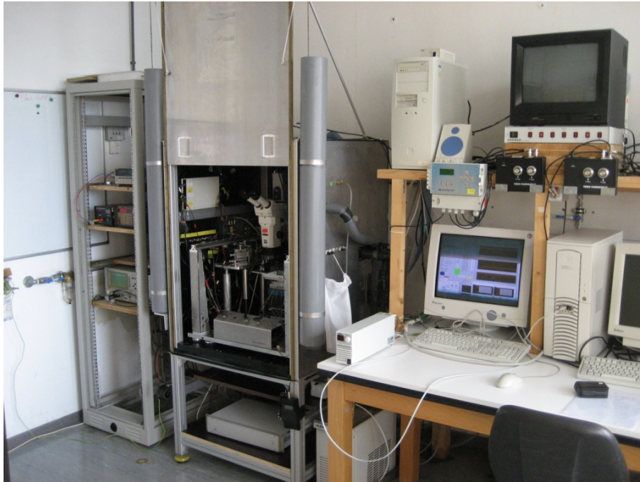
Figure 8.1: One of the two sensor teststations of the IEKP Karlsruhe. The station is used for the quality testing and the research on semiconductor radiation sensors. Operational elements of the sensors can get connected with different measurement devices and power supplies via relay stations to apply voltages and to fulfill measurements. A LabView software on a PC controls the devices and relays according to flexible user-defined test-programs.
