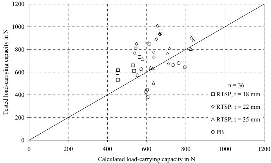
Figure 9 Tested load-carrying capacity vs. calculated load-carrying capacity for staples driven in directly
