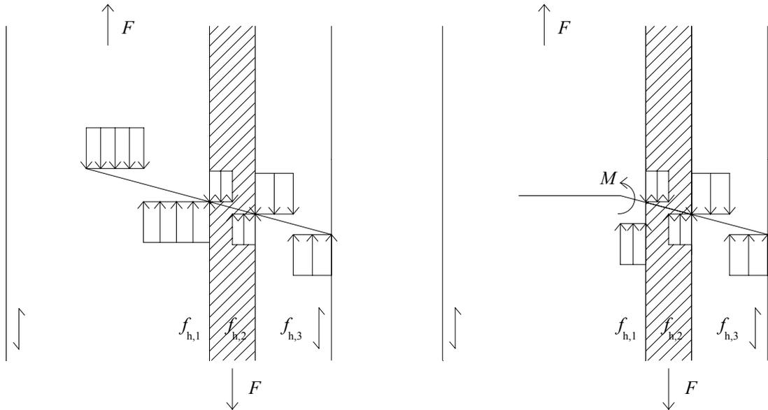
Figure 5 Extended failure modes 1a and 2b according to Johansen's yield theory
