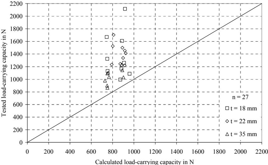
Figure 8 Tested load-carrying capacity vs. calculated load-carrying capacity for staples driven in through counter battens
