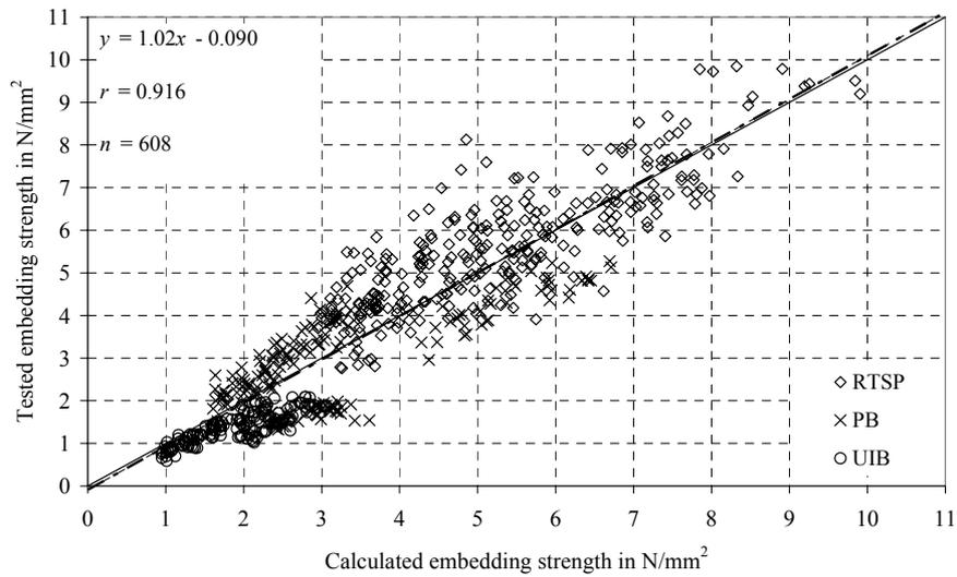
Figure 2 Tested embedding strength vs. calculated embedding strength
