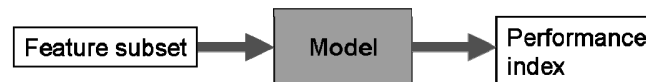
Fig. 1 Basis for the online monitoring is a subset of relevant features and a model which describes the impact of the features to a user-defined performance index. Both the relevant features as well as the model are derived from historical process data
