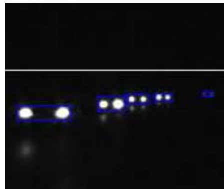
Figure 8 - Pairs of light sources grouped together by clustering algorithm. [3]
