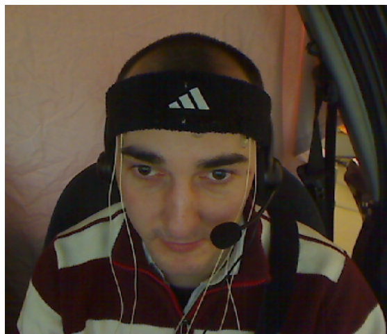
Image 2: (Part of) the recording setup with EEG headband and headset in the driving simulator
