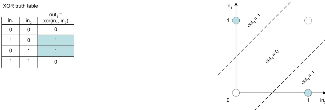
Figure 3.7: Logical XOR function. The truth table of the XOR function is shown on the left. On the right the input space \{in_1, in_2\} is plotted with the associated outputs out_1 . There exists no single hyperplane that can separate the areas with out_1 = 1 from the areas with out_1 = 0 .
