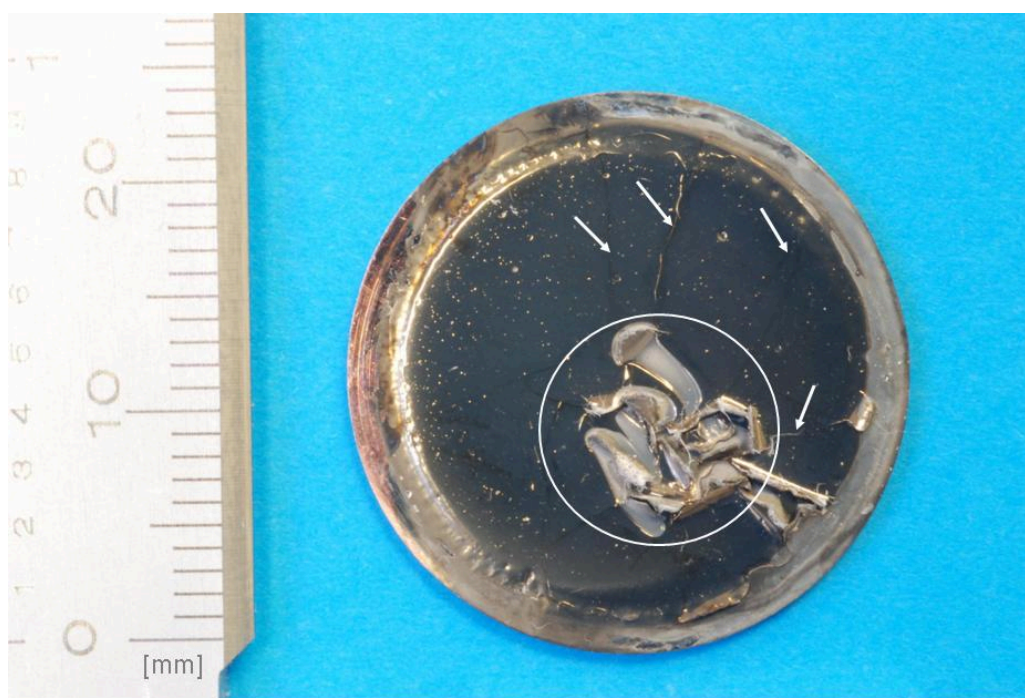
Figure 4.25: A Ni-Al 2 O 3 layer on copper substrate electrodeposited at a Ni 2+ concentration of 1.06 mol/L. Cracks at the surface are indicated by arrows. The circle surrounds a delaminated part. Underneath the latter electrodeposited Ni-Al 2 O 3 is observed.
