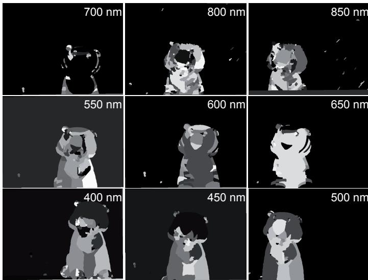
**Figure 5.4:** Segmented images from Figure 5.2 using the watershed transformation.
