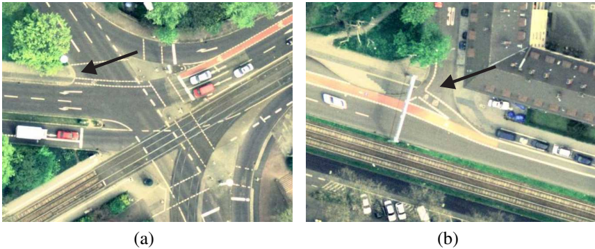
Figure 6.9: Intersections 9 (left) and 2 (right) classified inconsistent. The BicyclesOnlyLane which left the road network and therefore caused the inconsistency, is marked by a black arrow. (Source: City of Karlsruhe, VLW geo data)
